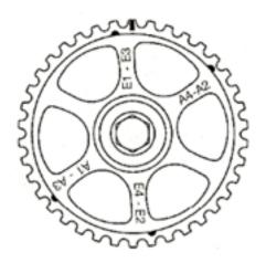
**1st Mark** | Exhaust 1 and Exhaust 3 **2nd Mark** Intake 1 and Intake 3 **3rd Mark** Exhaust 2 and Exhaust 4 **4th Mark** Intake 2 and Intake 4
